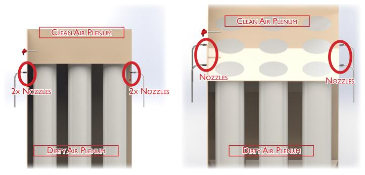
The images depicted below show the installation of CO2 nozzles and thermal probes installed on a dust collector with horizontally oriented filters. When available, CO2 nozzles can be installed on the side of the dust collector that is open to filter ends to allow CO2 nozzles to discharge down the length of the filters.
